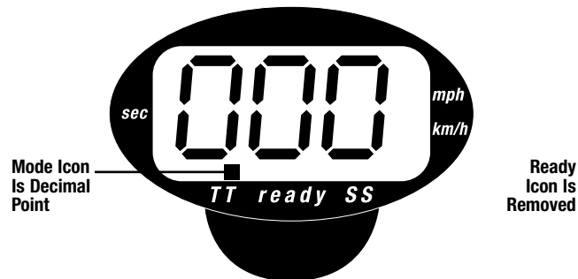
Figure 7 — Display at the Start of a Tempo Time Measurement
