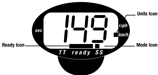
Figure 5 — Display Indication of SS Mode—km/h units
