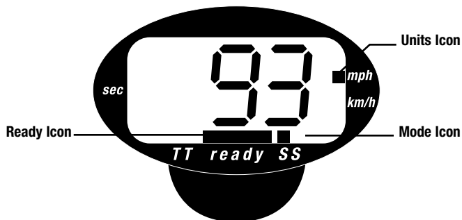
Figure 4 — Display Indication of SS Mode—mph units
