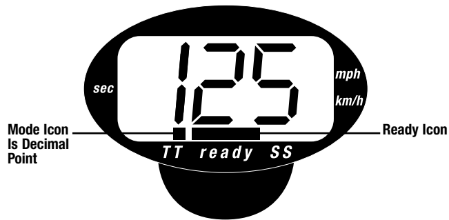
Figure 6—Display Indication of TT Mode
