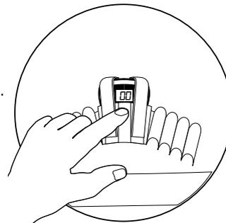
4. Press the Push-Button Switch a second time. **Two flashing zeros** indicate that the radar is transmitting. The KickSpeed Radar® is now ready for measuring the velocity of a ball approaching the Target.
