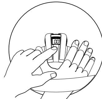
3. Just below the radar Display is a Push-Button Switch by which the KSR is powered “on”, as shown previously. **Press through the pouch to push the Button**, turning the radar “on”, energizing the radar Display. The KM/H Display will show the last reading.
