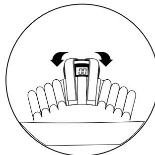
2. Place your right or left hand under the elastic Wrist Strap of the Target, and insert your fingers and thumb into the elastic Finger Loops. **The thumb and forefinger should span the radar pouch, as shown in the illustration.**
